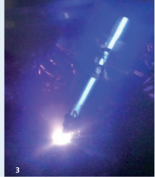
Pulsed electron beam for material ablation
